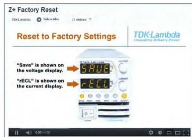
The first video produced by TDK-Lambda explains how to reset the Z+ back to its factory settings. This facilitates the sharing of these power supplies between several users and/or assists those who had initially set the unit incorrectly to modify the settings.
