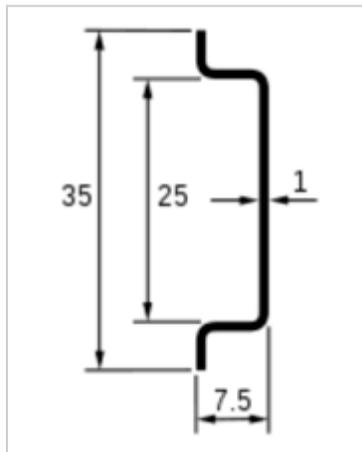
Figure #1 – End view of typical DIN Rail
