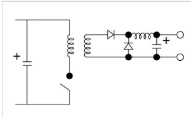
When a pulsed (peak) load is applied to the power supply in excess of its rated current, the energy is first drawn from the output capacitor. This can add to the capacitor ripple current, raising the temperature and reducing the component's life. Heat, as I explained in earlier blogs, dries out the capacitor's electrolyte.
