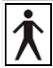
Type B (“Body”) is the least stringent classification, and is used for applied parts that are normally not conductive and can be immediately released from the patient. Examples of that would be LED operating lighting, medical lasers, MRI body scanners, hospital beds and phototherapy equipment.
