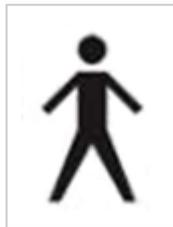
Type B applied parts may be connected to earth ground, but Type BF & CF are separated from earth – hence the term “floating”.
