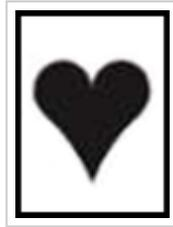
Type BF (“Body Floating”) is less stringent than Type CF, and is generally used for applied parts that have conductive contact with the patient, or having medium or long term contact with the patient. Examples of this type of equipment are blood pressure monitors, incubators and ultrasound equipment.
