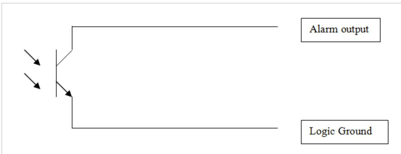
**Fig. B: This opto-isolated alarm signal has a separate output and ground**
