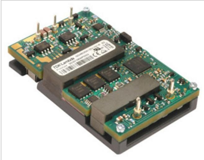
The “brick” style DC-DC converters are designed to be either conduction cooled (to a cold plate), or forced air cooled, often without an external heat sink. The rate of airflow available will depend on the user’s application, and so a number of performance curves are provided. It can be noticed that in some cases for low airflow conditions, de-rating has already occurred already at 30C ambient.
